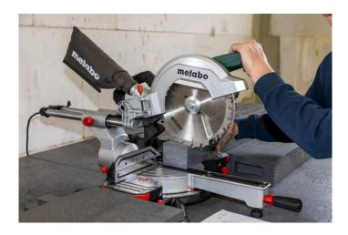
Recommended tool: Mitre saw with coarse longitudinal-cut blade (e.g. blaugelb HW Saw Blade 250x3.2/2.2x30 mm Z24 W item no. 0399564).
