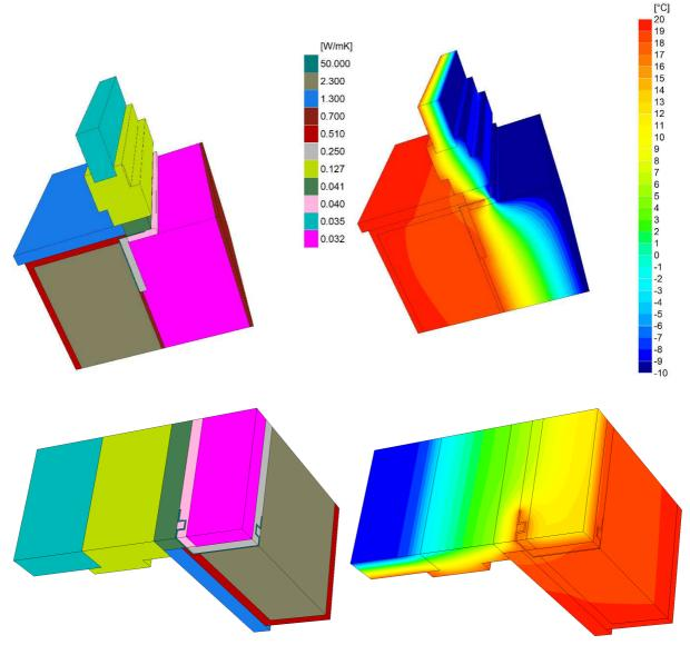
Figure 3: Bottom connection: extracts from the 3D models. Left: materials, right: isotherm view.
