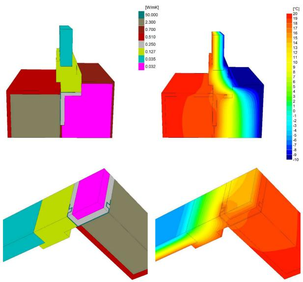
Figure 4: Side and top connection: extracts from the 3D models. Left: materials, right: isotherm view.
