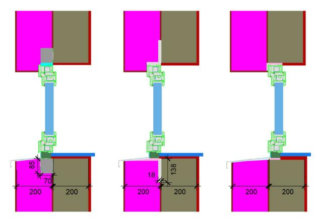
**Figure 1:** 2D models of the installation situations. Left, with blaugelb Trio**therm**<sup>+</sup>. Centre, for installation with steel angles. Right, flush with the wall.
